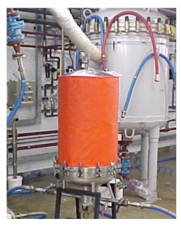
Outer surfaces of each jacket utilise tough, water resistant nylon materials, inner layers are manufactured using unique coated glass cloths for protection from chemicals and long-term temperature durability. All heating jackets utilise high efficiency insulation to reduce heat-loss to a minimum, therefore we can also provide unheated insulated covers to fit containers where electrical power is not required or not available.
